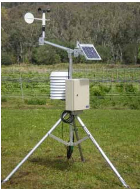
*A recently installed Automatic Weather Station*
