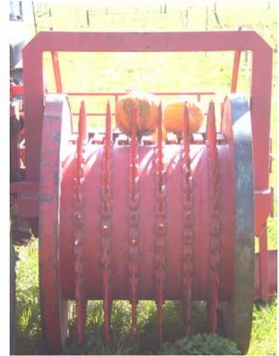
*One section of the specialised 'harvester' being used in the current Myrtleford trial. The mature pumpkins are 'picked up' by the machine. The harvester also separates and retains the seed and expels the pumpkin flesh which can be used as stock fodder.*
